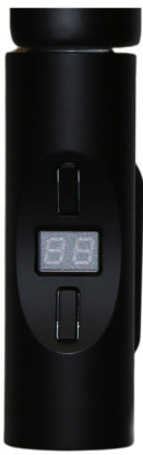
Temperature Regulating Element- Digital screen to set the temperature from 10-65 degrees. Turbo mode to set max temperature for 1-3 hours. Timer mode to set desired number of hours for heater to be on (up to 9 hours)
